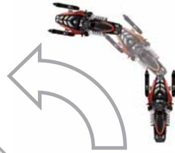
Sled turns like it's on rails. Amount of turning carbide on skis is balanced with the number of track studs.
