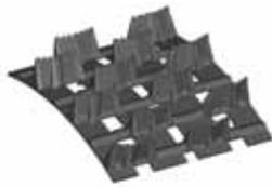
» Industry leading deep powder track. For 8T Drive sprockets, 2.86" pitch. Available in 146," 155" and 163" lengths.
