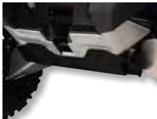
Front mount does not reduce clearance and can be installed with or without front skid plate.
